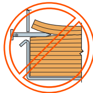
Nail at Wrong Angle
